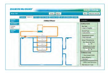
A variety of cooling plant system types and configuration can be compared in EnergyAnalyzer II to select the system that meets performance and cost requirements.
